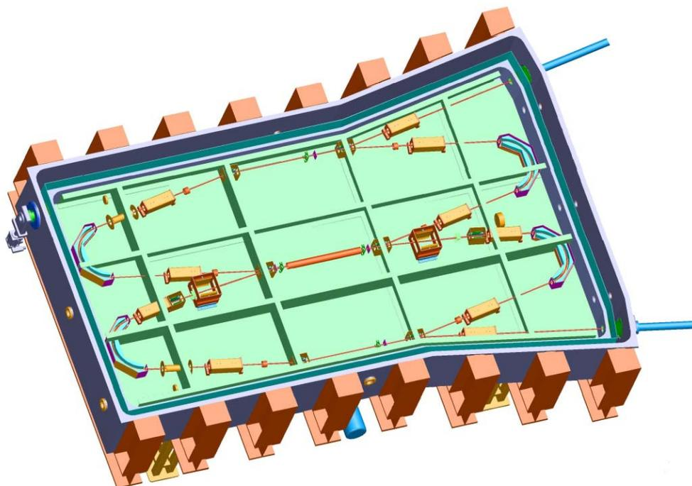
Fig.1. Schematic layout of DESIREE with the lids of the vacuum vessels off. The outer dimensions are approximately 5×3×1 m.
