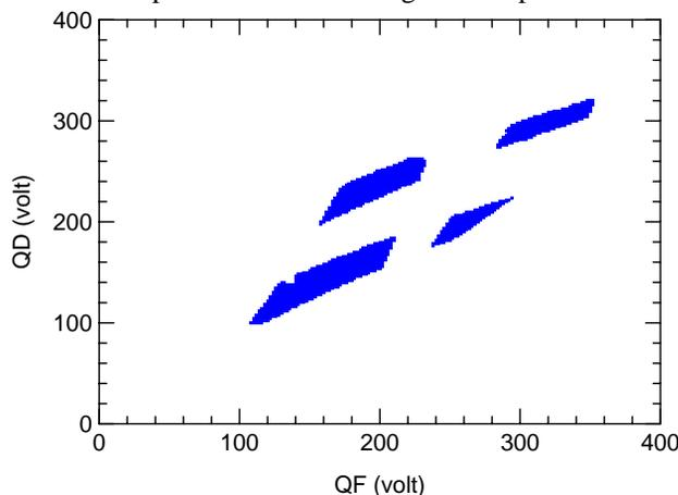
Fig. 2. Areas of stable motion in ring 1 as a function of the two quadrupole voltages, assuming 10 keV ions.
