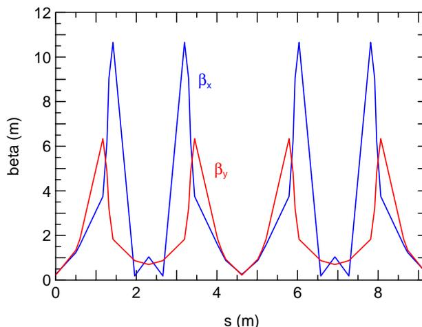
Fig. 3. Example of beta functions in ring 1 at a working point where the beam has a focus in the straight sections.
